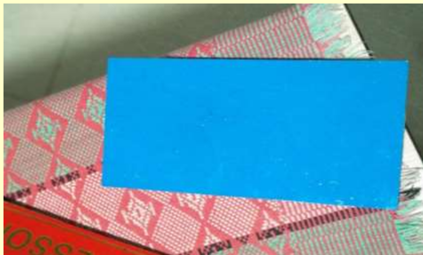
ECO friendly Manufacturing of Tiles from used PET Bottles
